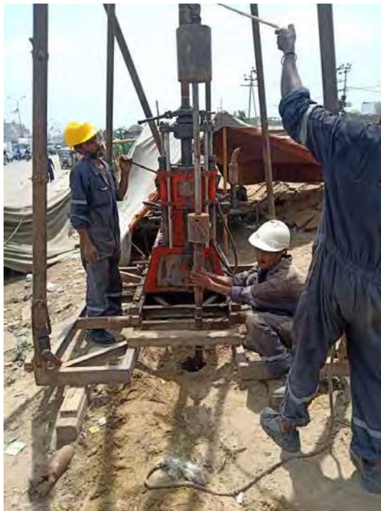
Plate-2: Performance of Standard Penetration Test (SPT)
