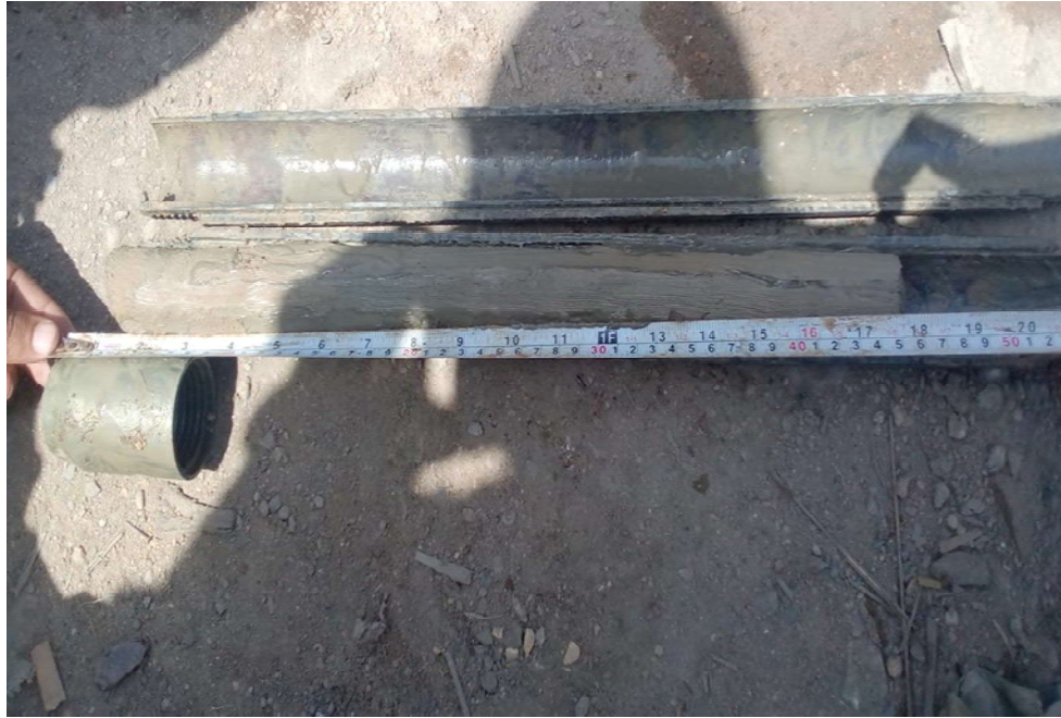
Plate-3: A View of Soil Sample Recovered in Split Spoon Sampler
