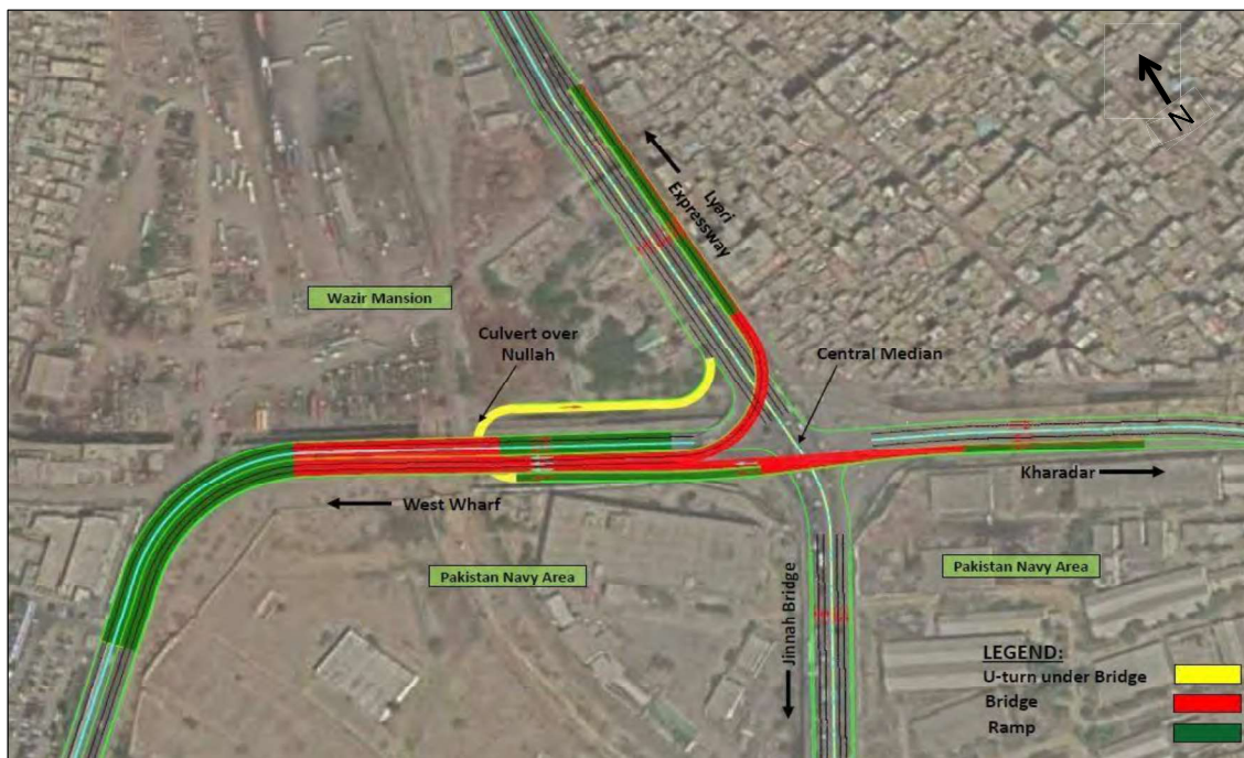
Figure 4.1: Option II - Flyover on Mauripur Road & Kharadar with grade U-turn under ICI Bridge
