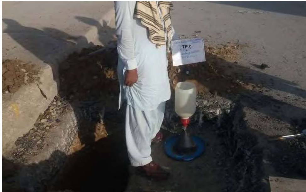
Plate-4: Performance of Field Density Test in Base Course Layer
