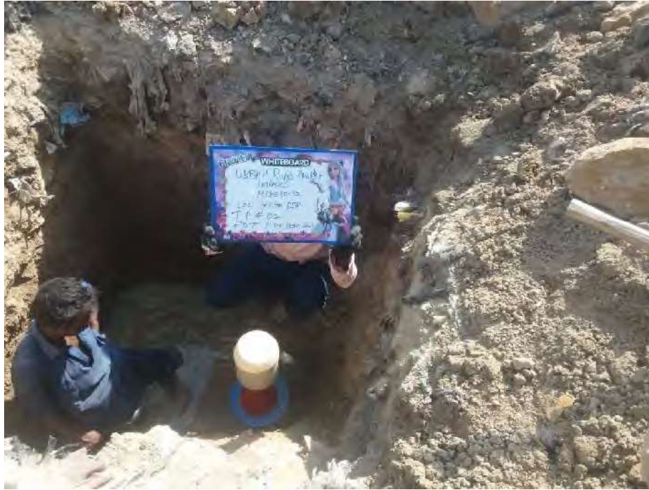
Plate-5: Performance of Field Density Test in TP-02
